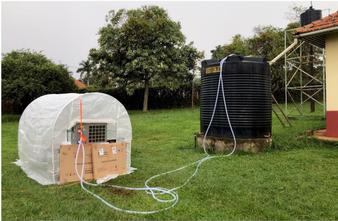
Figure 1. The drying enclosure with the heat pump in position in the eastern end (gaps yet to be closed), the 10,000-L rainwater tank, and the pipe along which water was pumped from the tank to the heat pump. Source: Authors
