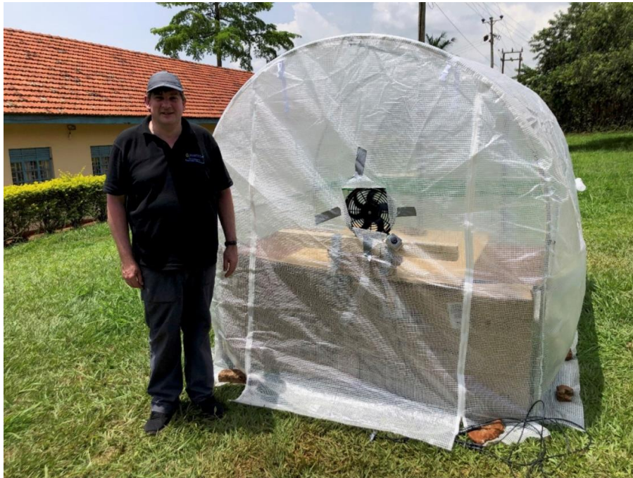
Figure 3. The drying enclosure as used in Experiment 2 on February 25, with a simple fan in place of the heat pump used the day before in Experiment 1. The fan delivered air at the same rate that the heat pump had, but the fan diameter was smaller so fan speed was higher.
